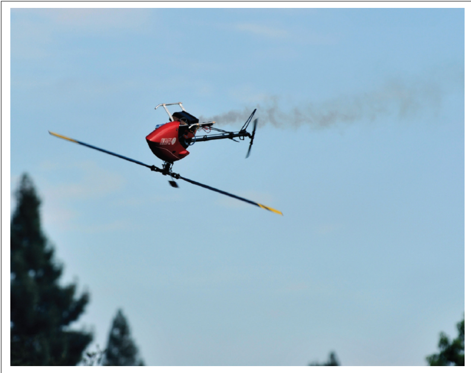
Figure 8-4. Andrew Ng's team at Stanford, from 2004 to 2010, trained a helicopter to learn to fly upside down using reinforcement learning. This work required the construction of a sophisticated physically accurate simulator.
