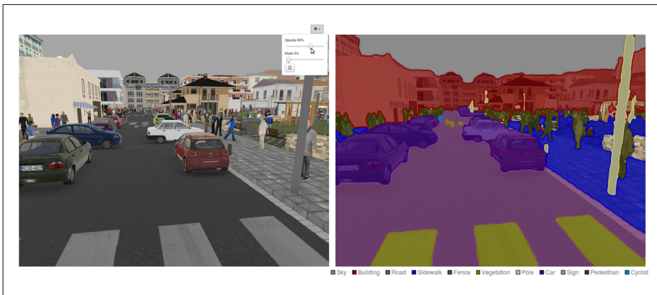
Figure 6-10. Objects in an image are “segmented” into various categories. Image segmentation is expected to prove very useful for applications such as self-driving cars and robotics since it will enable fine-grained scene understanding.
