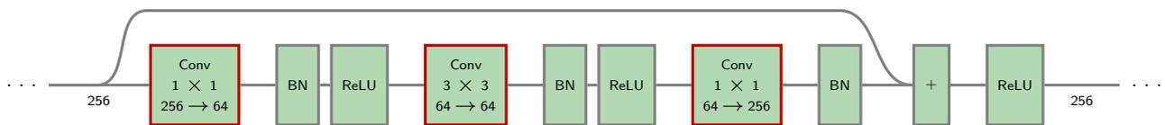
$$256 \times 64 + (3 \times 3 \times 64 + 1) \times 64 + 64 \times 256 \simeq 70k \text{ parameters.}$$
