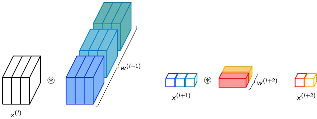
This “convolutionization” does not change anything if the input size is such that the output has a single spatial cell, but it **fully re-uses computation to get a prediction at multiple locations** when the input is larger.
