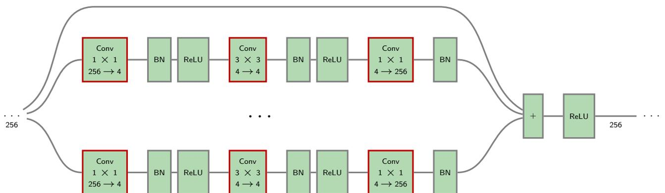
When equalizing the number of parameters, this architecture performs better than a standard resnet.
