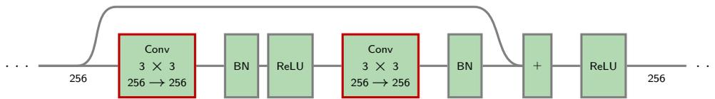
However, such a block requires  $2 \times (3 \times 3 \times 256 + 1) \times 256 \simeq 1.2m$  parameters.
