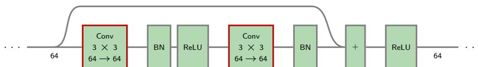
and as such requires  $2 \times (3 \times 3 \times 64 + 1) \times 64 \simeq 73k$  parameters.
