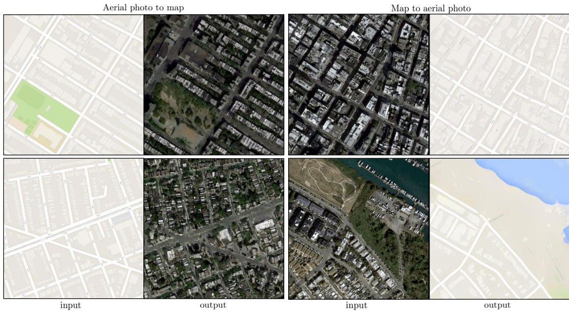
Figure 8: Example results on Google Maps at 512x512 resolution (model was trained on images at 256x256 resolution, and run convolutionally on the larger images at test time). Contrast adjusted for clarity.
