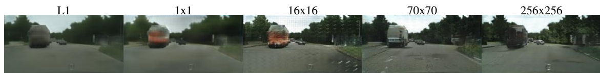
Figure 6: Patch size variations. Uncertainty in the output manifests itself differently for different loss functions. Uncertain regions become blurry and desaturated under L1. The 1x1 PixelGAN encourages greater color diversity but has no effect on spatial statistics. The 16x16 PatchGAN creates locally sharp results, but also leads to tiling artifacts beyond the scale it can observe. The 70x70 PatchGAN forces outputs that are sharp, even if incorrect, in both the spatial and spectral (cofornfulness) dimensions. The full 256x256 ImageGAN produces results that are visually similar to the 70x70 PatchGAN, but somewhat lower quality according to our FCN-score metric (Table 2). Please see https://phillipi.github.io/pix2pix/ for additional examples.
